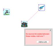
These drainage links are made by selecting "water supply" in the viewing options, and then left click and hold on the source node and then release the hold over the demanding node. This will raise a further options window, firstly checking whether a link already exists, and then if you add a link, leads to a request to input the priority and weight of the link.
