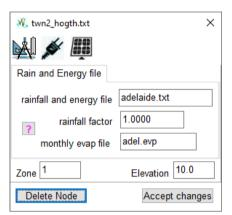
To modify the parameters in each of these nodes select Model Components from the right-hand menu and then left click on a node currently in the layout. This raises the base window shown adjacent.
